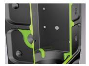
thickened cross-sections applied in the places of increased stresses
